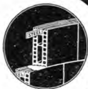
Natco Silo Wall. Note perforated shell, providing firm anchorage for mortar joints.
